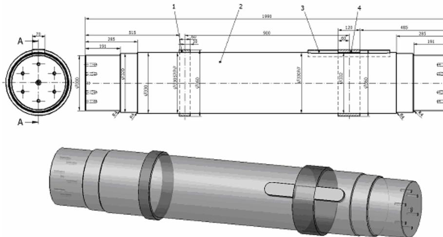
**Fig. 6.** Modified pulley shaft at Lonea Mining Plant
