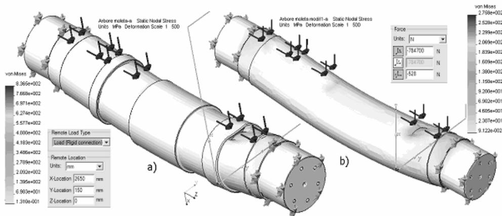
Fig. 7. Analysis with finite elements of the two shafts, existing and proposed
