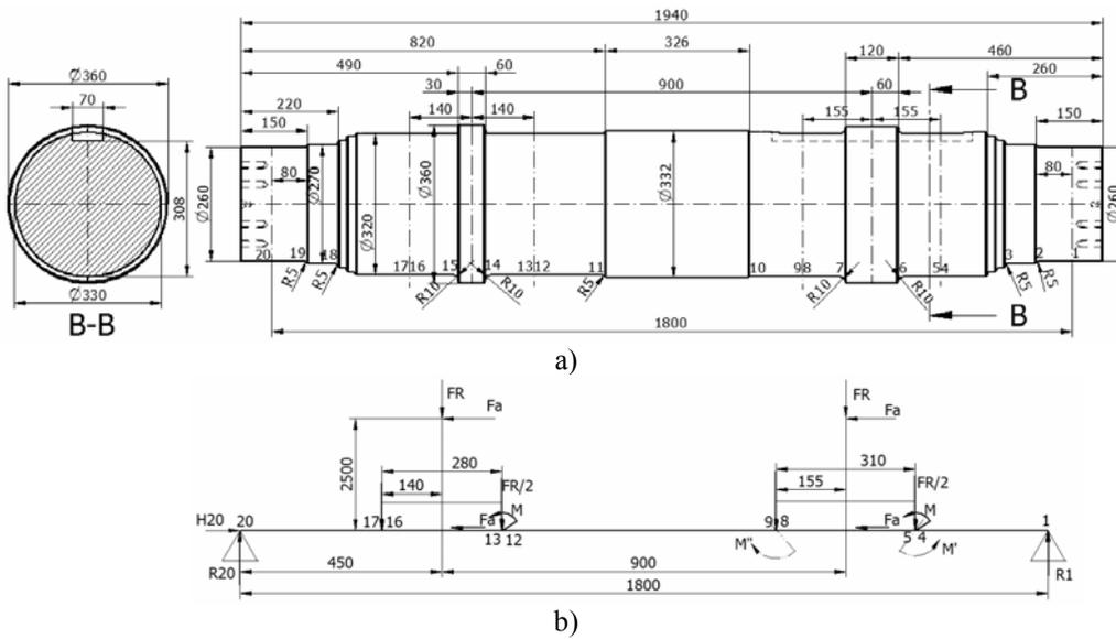
Fig. 3. Shaft design size and mathematical load model
